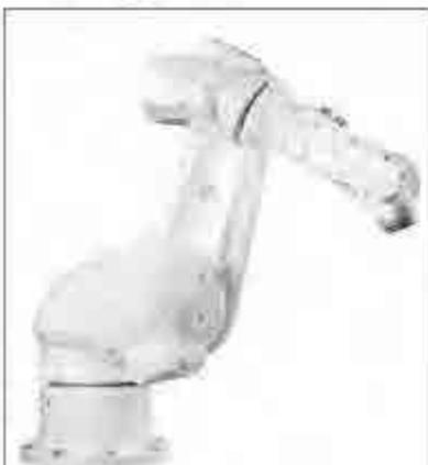
Robot designed for humid food processing environments, courtesy Stäubli Corporation
