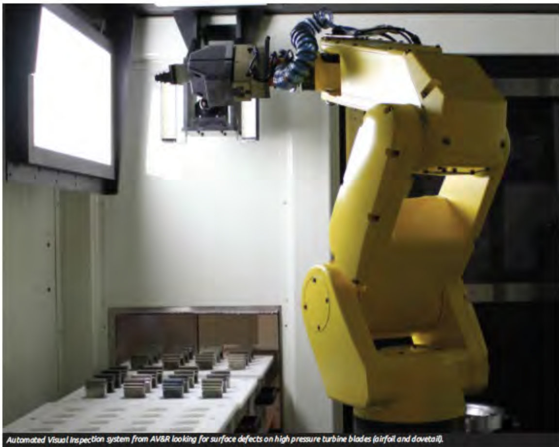
Automated Visual Inspection system from AV&R looking for surface defects on high pressure turbine blades (airfoil and dovetail).
