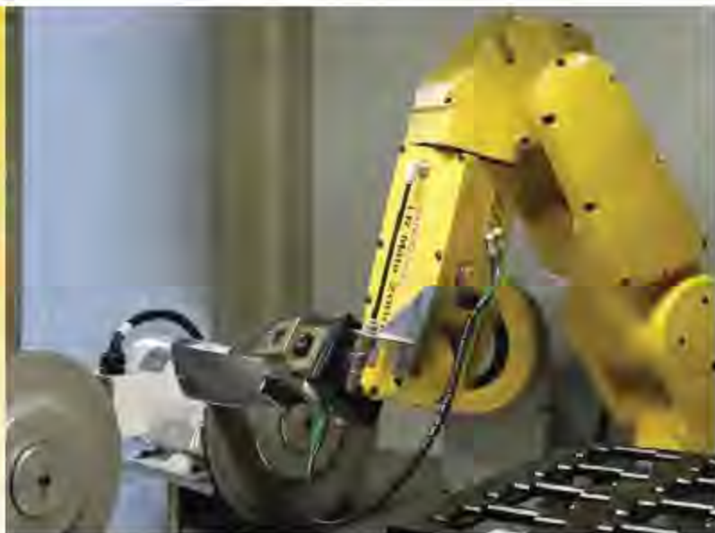
This automated blade profiling system integrates all the required abrasive wheels needed to perform the profiling.
