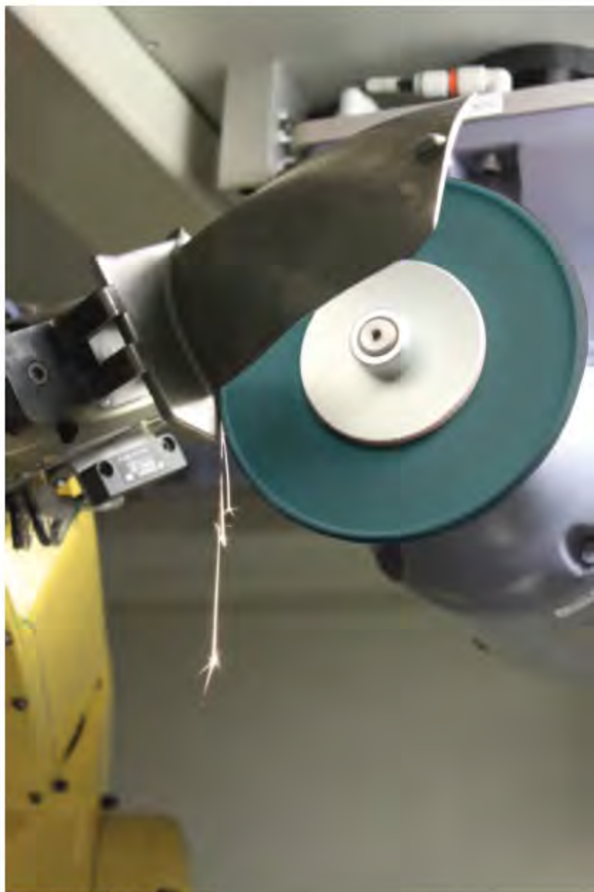
AV&R's automatic blade blending system.
