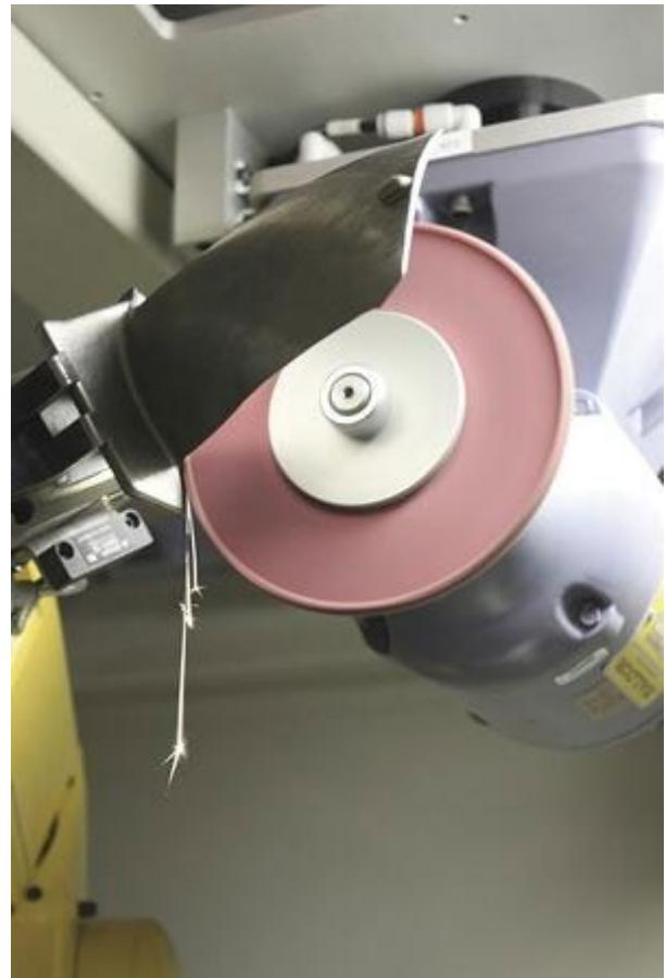
Jet engines are high performance machines and a burr, even if it is only one thousandths of an inch, can have expensive and dangerous consequences. Each turbine blade within the engine must be manufactured to tight tolerances. These blades routinely operate under high stress, and edge breaking is a method used to strengthen the components. When a micro radius is put on a part to spread the
